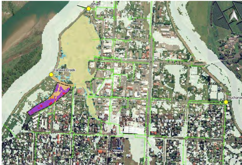
Figure 0-7 : Areas of surface flooding in Opotiki Township for 10% AEP
