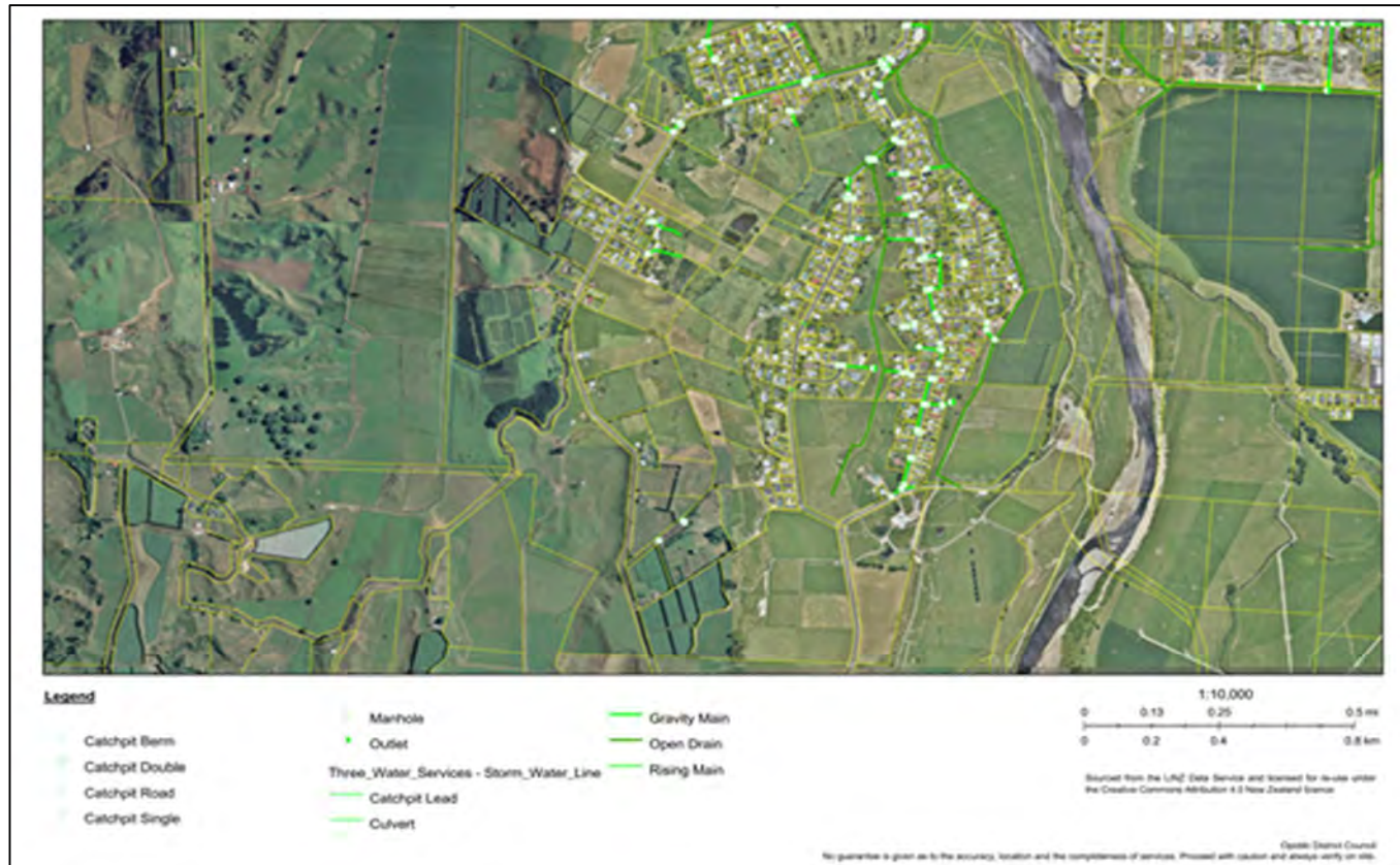
Figure 3.9 Hukutaia– Stormwater Provisions.
