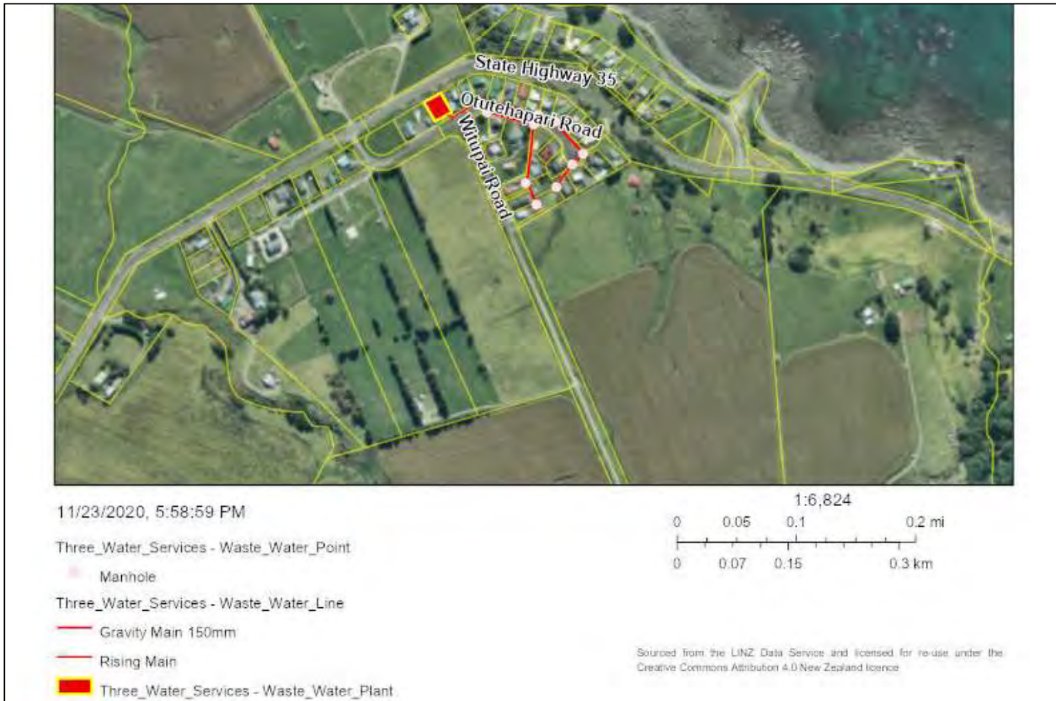
Figure 3 6 Wastewater network in Waihou Bay.
