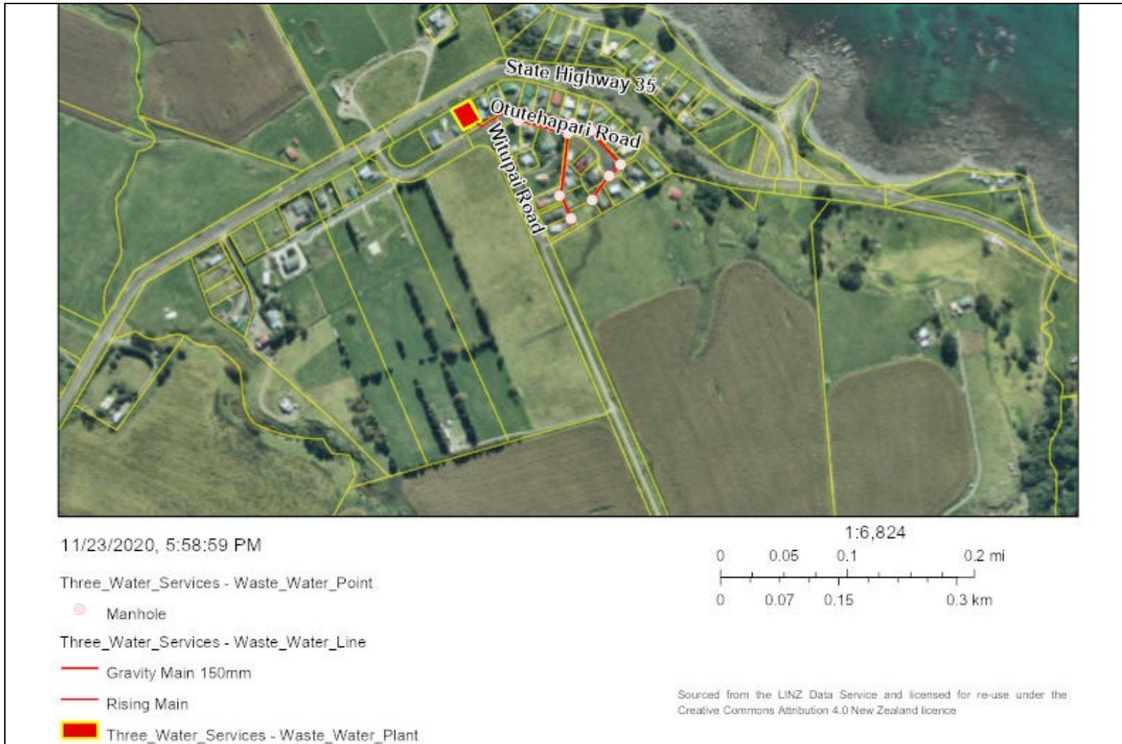
Figure 3 6 Wastewater network in Waihau Bay.
