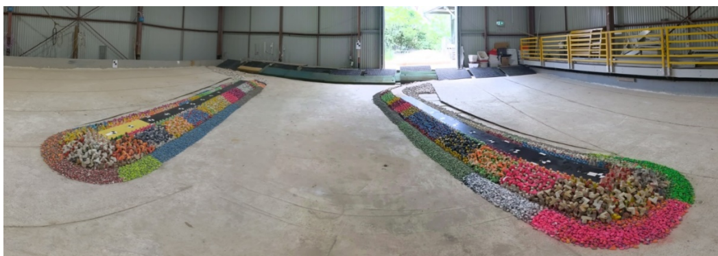
Figure 5-3: Physical model constructed in a wave basin to validate nearshore wave heights and training wall structures' influence on wave climate.
